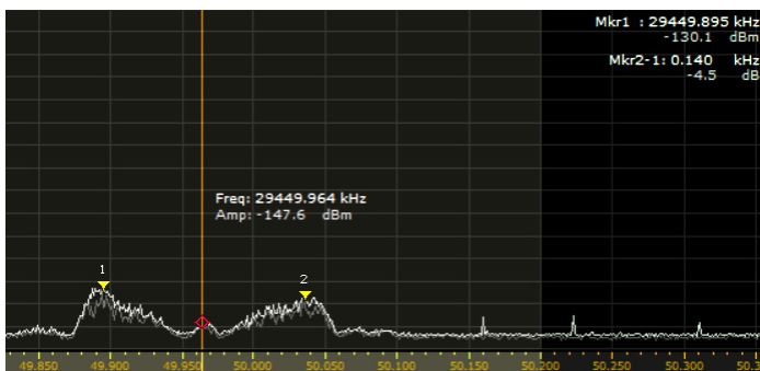
FSK; 81.9Bd; Shift 140Hz; Ocean data measurement buoy
